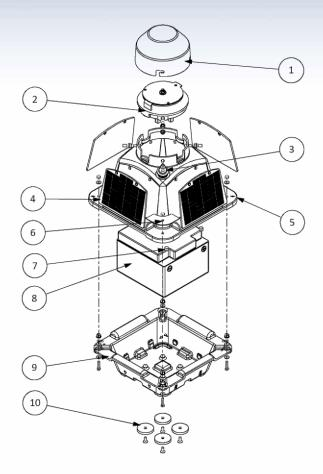
1. Optical glass 2. Resin-coated electronics 3. Push button 4. Solar panel 5. Body 6. Identification plate 7. Battery protection covers 8. 12V Battery 9. Base
